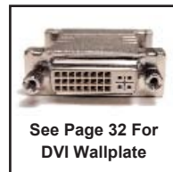
35-710 DVI-I to DVI-I Female to Female Inline Coupler. Shielded di-cast case handles 5 pin analog and 24 pin digital signals. gold plated contact pins. Used for inline or chassis mount. Fits in standard DB15 d-sub cutout. Overall length .93" For wall mounting use Calrad p/n 30-598
