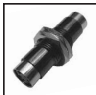
35-498 4 pin 35-498-6 6 pin 35-498-8 8 pin 35-498BC Black Chrome Bulkhead SVHS connector with 2 nut mounting. Panel mount 4 pin SVHS female to female. Mounts in 1/2" double "D" hole.
