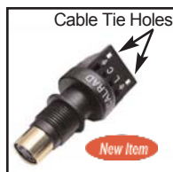
Cable Tie Holes 35-498K-S Solderless Keystone or chassis mount SVHS jack with screw terminal connectors. Mounts in 1/2" hole or standard keystone insert. Comes with cable tie for strain relief. Colored ID washers available (30-288-COLOR). Also available in BNC (75-686K-S) and RCA (30-308K-S) versions.
